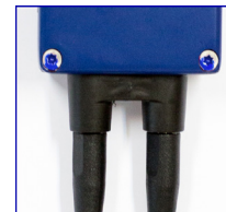
VIII. Check if CLC is closely attached to Main Box (no space between both objects)
