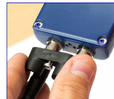
II. Remove Connectors Locking Clip (CLC)
